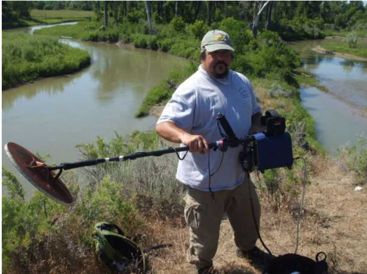
Figure 3. Chris Adams holding the Minelab GPX 4000 pulse induction metal detector. Note the operator must be as metal free as possible to deploy the machine. The battery is carried in a separate case strapped to the back of the operator.
